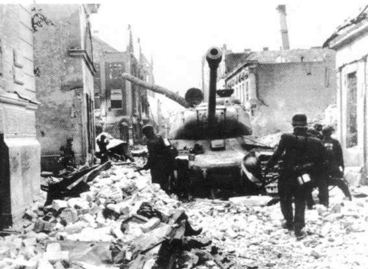
Above: Waffen-SS troops pass a knocked-out Russian JS-2 heavy tank on the Eastern Front in spring 1944. The most powerfully armed tank in the world at the time with a 122mm main gun, the JS-2 entered production in late 1943.
