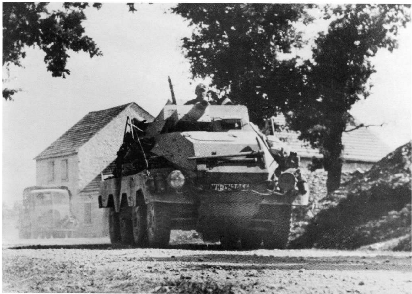
Above: SdKfz 233 heavy, eight-wheeled armoured car. Main armament is a short-barrelled 75mm.
